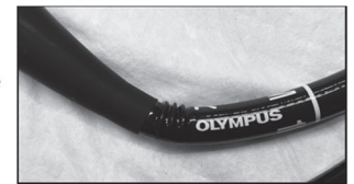
Photo courtesy Ofstead: Scope with buckled insertion tube
