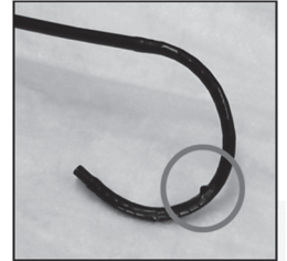
Photo Courtesy Ofstead; Ureteroscope with damaged bending section
