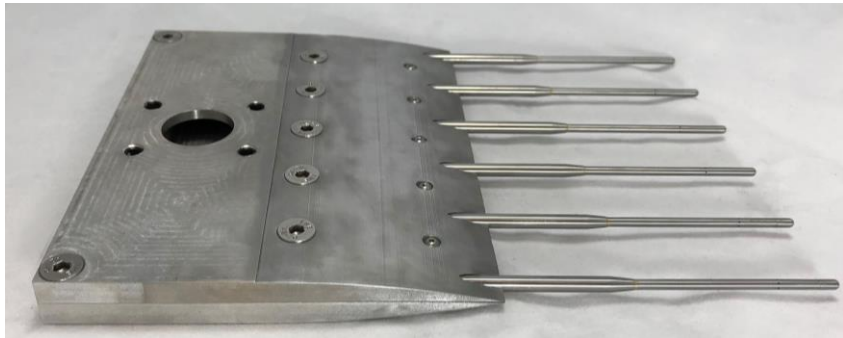
5-Hole Probe Rake with 3 tips, 1.6 mm diameter probe tips.
