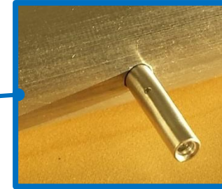
Kiel rake for thrust reverser measurements, 1 meter long.
