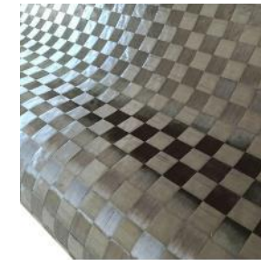
Spread tow fibres offer <50gsm fabrics
